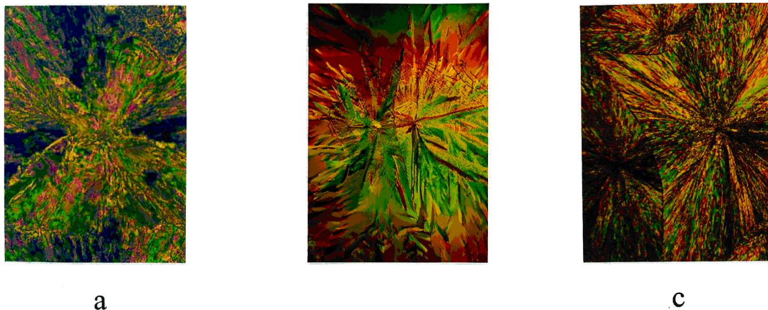
Figure 3. Optical textures of three bis( \beta -diketonato)copper(II) complexes: (a) C_6 EDK-Cu ( 140^\circ\text{C} ); (b) C_{11}C_{12} DK-Cu ( 120^\circ\text{C} ); (c) EEDK-Cu ( 94^\circ\text{C} ).
